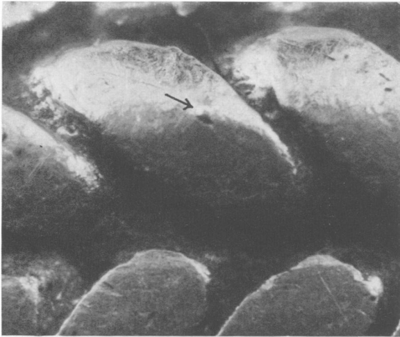
c. Platinum metal inclusion on twisted wires of Egyptian ring shank. Late 2nd mill. B.C. \times 100
